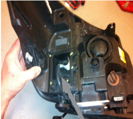
Ford provided side marker mounting platform on rear of headlight assembly.
