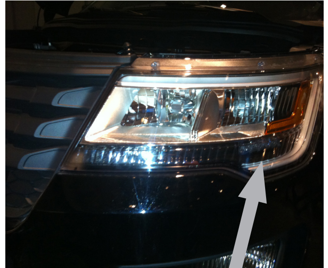
MARKER LIGHT INSTALLATION LOCATION
