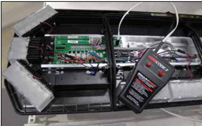
**Quick:** Clone an existing lightbar flash pattern configuration with a hard wire connection from the lightbar to the SmartPro that allows you to copy the flash patterns to multiple lightbars.
